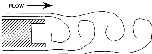
Fig. 1 Typical two-dimensional base cavity and subsonic vortex street wake.
